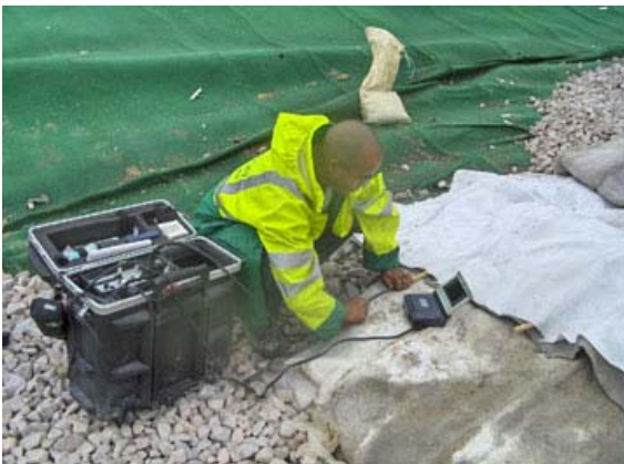
Figure 6. Insertion of the endoscope into the mini-pipe
