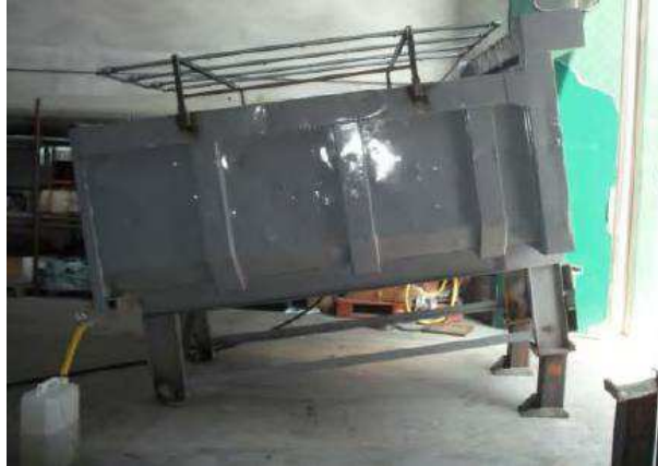
Fig. 13. Inclinable open box with a rainfall simulator
