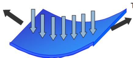
Figure 2: Illustration of membrane effect
