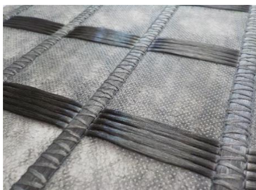
Figure 1. The Notex® Glass geosynthetics are obtained by warp-knitting a light geotextile and a glass-fiber geogrid. An additional coating can also be added when needed (here, with bituminous coating).
