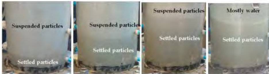
(a) after 5 minutes (b) after 15 minutes (c) after 2 h 45 min (d) after 66 hours Figure 8 Settlement of the slurry during the first stage of the test
