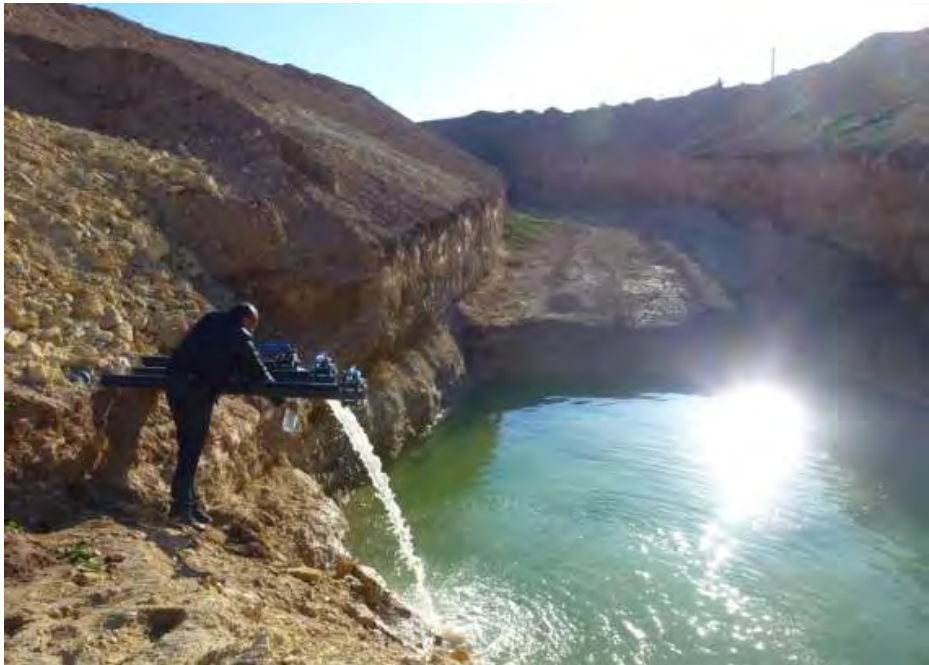
Figure 15: system in operation – Collected water from the bottom on the test pond
