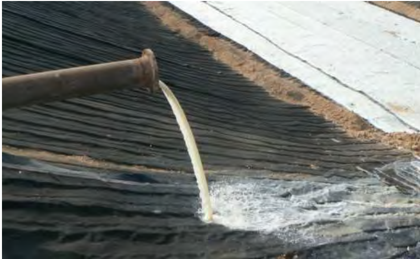
Figure 13: multi-linear drainage geocomposite used in a slurry dewatering facility (photo courtesy Afitex- Texel)
