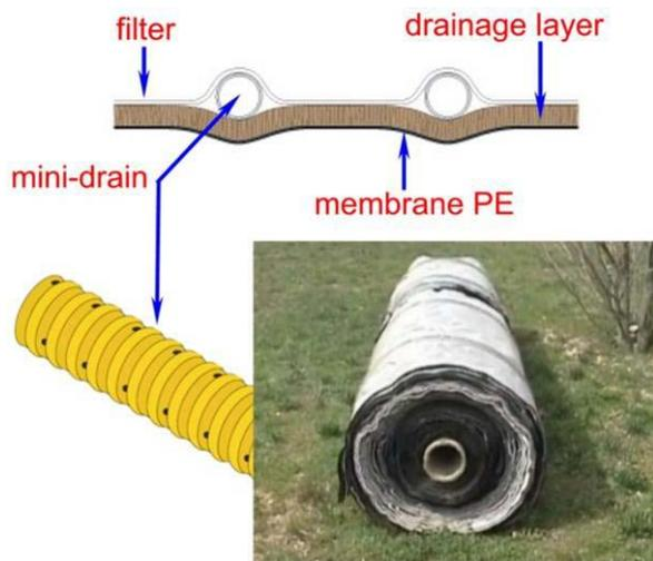
Figure 2. Geocomposite DRAINTUBE FT/PE structure
