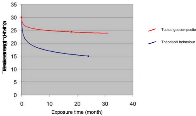
Figure 7. Loss tensile strength of the geocomposite installed in Villeparisis versus exposure time
