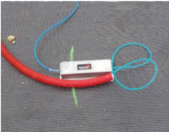
Figure 13. Hydraulic settlement gauge
