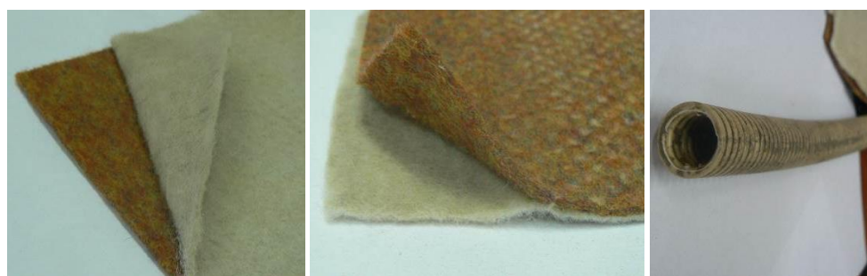
Fig. 7. Visual inspection of the exposed geocomposite (geotextile layers and mini-pipes).
