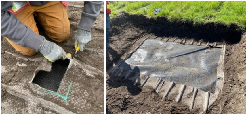
Fig. 10. A large sample is collected to be sent for laboratory testing.
