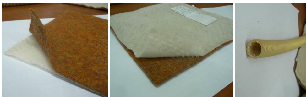
Fig. 6. Visual inspection of the virgin geocomposite (geotextile layers and mini-pipes).
